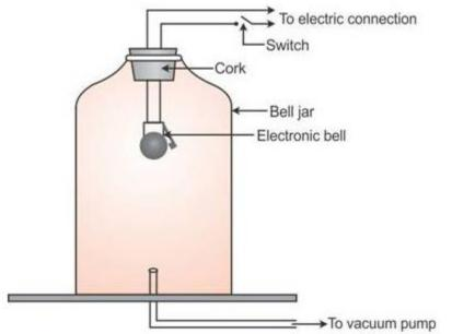
An electric bell is suspended inside an airtight glass bell jar. The bell jar is connected to a vacuum pump as shown in figure. As the circuit of electric bell is completed by pressing the key, the hammer of the electric bell begins to strike the gong repeatedly due to which sound is heard.
