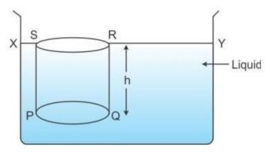
Total thrust exerted on the surface PQ
