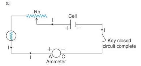
(c) A rheostat is used to control the current in the circuit.
